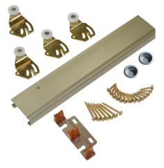
An economical prefinished gold colored steel bypass track with convex track rails, which provide one point contact between wheel and track. One wheel (7/8" dia.) hangers with three point locking. One inch high woodtone adjustable door guide. Brass-tone steel parts.
