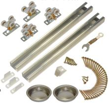
A commercial grade bypass sliding door hardware set for doors weighing up to 150 pounds each. Heavy-duty extruded aluminum box track utilizes three-wheeled ballbearing rollers (#1025) with 3/4" diameter machine turned wheels. The three piece guide is adjustable for different thicknesses of doors. (minimum door thickness is 3/4")
