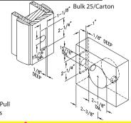
**2800F** Double Fascia Open Pocket Door Hardware for a 1%" to 134" Thick Door to 75 lbs.
