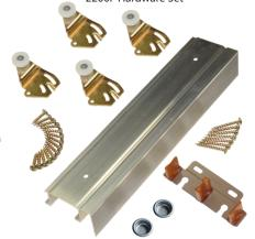
An aluminum fascia track with "Hi-Lite" design to hide blemishes that may occur. Convex track rails that provide one point contact between wheel and track. Hangers include one or two wheels (7/8" dia.) with three point locking. Hangers adjust without removing or relocating screws. Woodtone guide adjusts laterally for quick plumbing. Nylon guide posts are 1" high, guide posts swivel to allow warped doors to operate without binding. Brass-tone steel parts.
